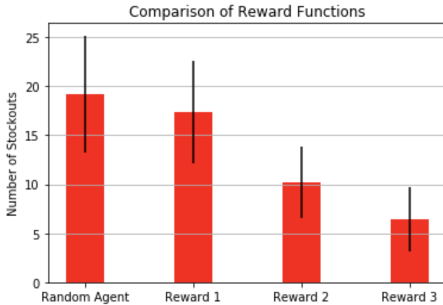
Figure 7.4: The bar graph show the number of stockouts obtained per episode averaged over 100 episodes. It illustrates the importance of reward shaping. The configuration 1 is used, the same as is used in Figure 7.1.
